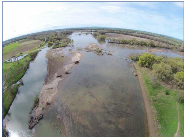
Targeted levee breaches, creating drainage swales, and lowering the floodplain for more frequent inundation, improved connectivity between the Cosumnes River and its floodplain.
